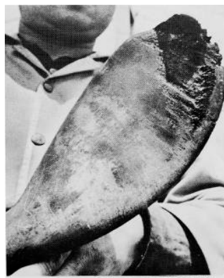
Corroded boat propeller in the city's toxic waters
